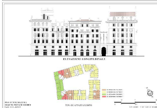
Shauni Priyam Sikder - Mixed residential block on the main square. Square elevation, Side elevation and subdivision of buildings and apartments.
