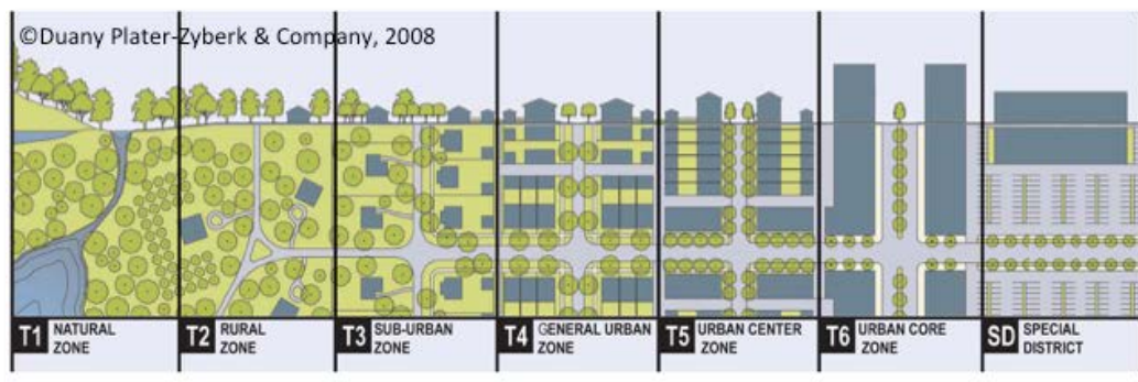
Figure 8: The current standard diagrammatic representation of the prototypical rural-to-urban transect.
