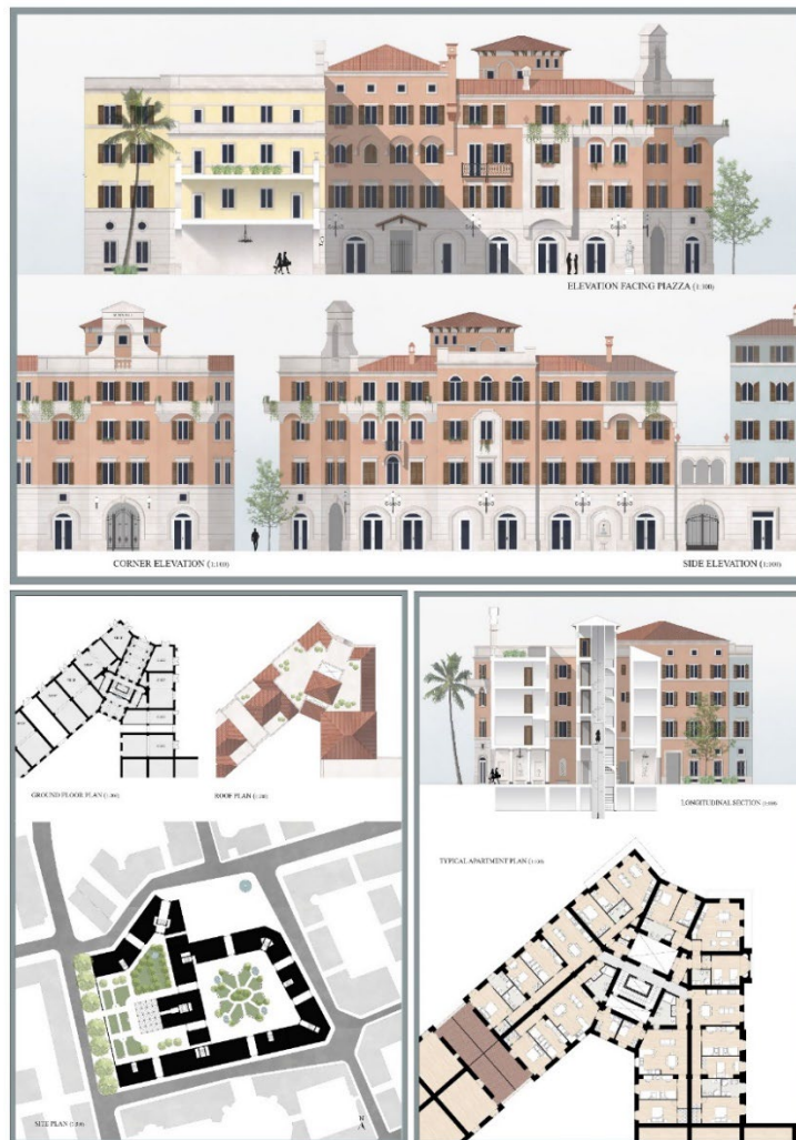
Alessandra Giannasca - Mixed residential use block - Insertion plan, floor plans and section
