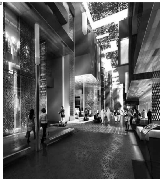
3. Climate as a determinant of design: a narrow shady street that channels breezes in Foster + Partners' design for Masdar City, Abu Dhabi
